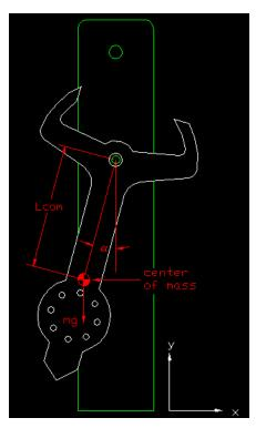
Fp = tension force in pendulum Lcom = effective length of pendulum mg = gravitational force on pendulum  $\alpha$  = angle between Fp and mg
