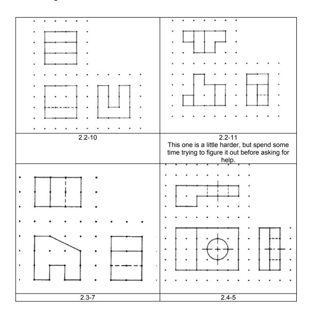
2. Construct a Orthographic 3-view sketch of each problem shown below. One problem per sheet and include your name, section number and drawing number on each sheet.
